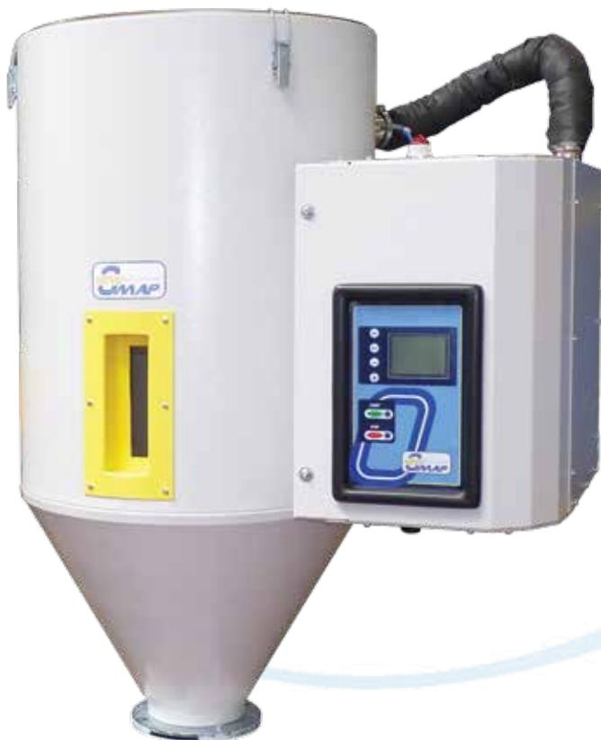
The Wheel Dryer WD series with honeycomb rotor has its new models **WD15-30** designed to be fitted directly on the drying hoppers ranging from 30 to 100dm<sup>3</sup> to have very compact and efficient solution machine-mounted.
