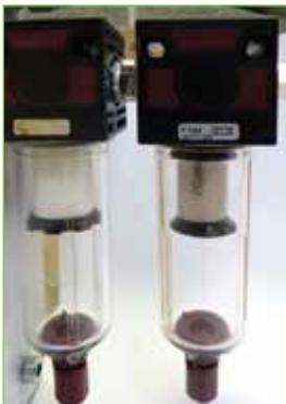
Extra filters to be placed at compressed air inlet for extra filtration, also available with pressure gauge to check and control line pressure.
