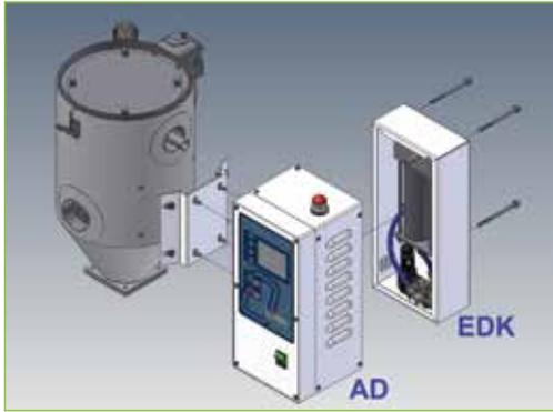
Extra drying kit, enabling the AD dryer to reach a working dew point of  $-50^{\circ}\text{C}$ .
