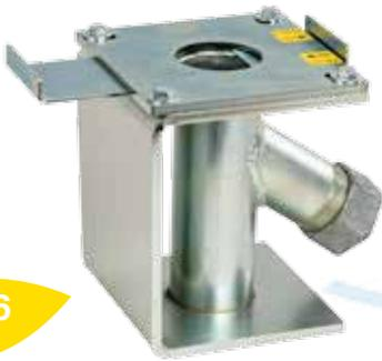
Supporting base for easy installation of dryer on machine throat, comprehensive of manual sliding gate and side discharge outlet for fast cleaning.
