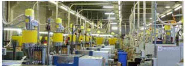
All our systems are pneumatically operated by vacuum and use the "starvation" method. The brain of the system is the microprocessor which transmits and receives data and safely controls the whole installation; it can be connected to any PC by serial port.
