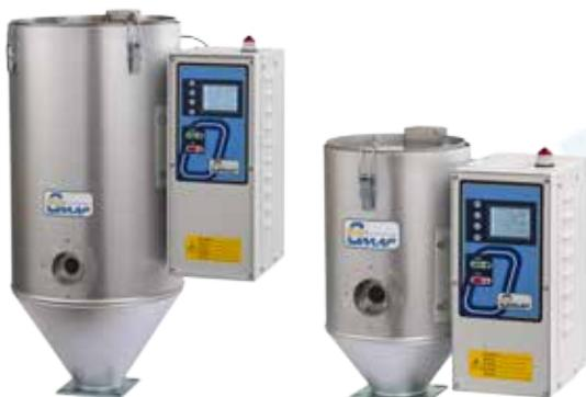
Using only compressed air, the **AD** series of dryers have a working dew point values of -20°C. With the addition of the "Extra Drying Kit" the **ADK** module, has a working dew point of -50°C. Suitable for small to medium throughputs.
